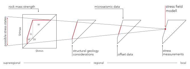
^ Basic workflow for stress tensor modelling. Starting from basic rock mechanics the possible stress states are defined and subsequently narrowed down by incorporating available data on your project area.
